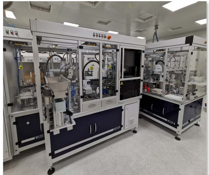
Device for automatic installation of FI relays
